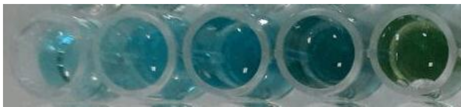
Fig. 6s. Colorimetric investigations of different concentrations from substrates (TMB and H 2 O 2 ) (low concentrations to high concentrations: from left to right) using Fe 3 O 4 /MWCNTs
